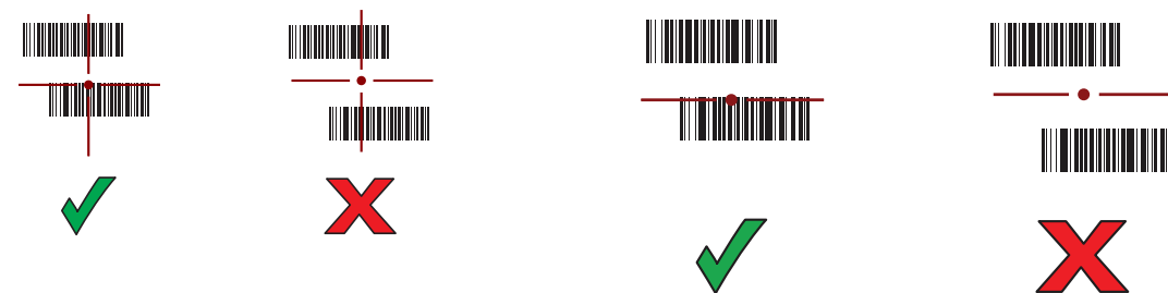
Figure 79 Pick List Mode with Multiple Barcodes in Aiming Pattern: Standard and Extended Range
