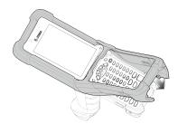
**4.** Turn the device over and ensure that the two alignment tabs completely fit into the two alignment slots on the device.
