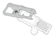
Grasp the bottom of the rubber boot and place over the bottom of the device.
