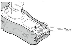
**NOTE** To charge the device in a cradle, completely remove the rubber boot.
