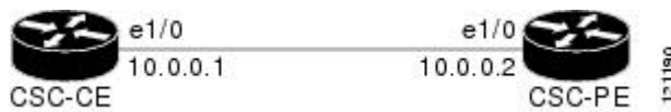
Figure 136: Configuration for Peering with Directly Connected Interfaces Between CSC-PE and CSC-CE Routers
