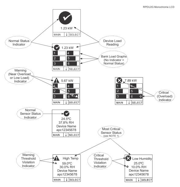
**NOTE 1:** The simplified LCD pages will show device load alarms only when no banks are present OR bank load alarms only when banks are present. Phase and Outlet alarms and warnings will NOT be displayed.
