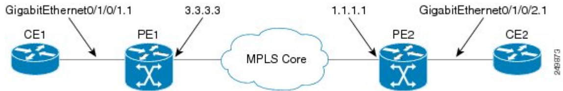
Figure 38: VPLS with BGP autodiscovery and BGP signaling
