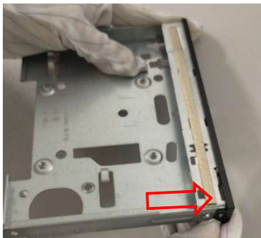
Figure39 Uninstall the left side and right side of the switch card cage.
