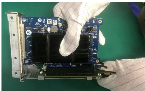
Figure15 Use PH1 screwdriver to uninstall the screws and Z4 G5 Rack DSR.
