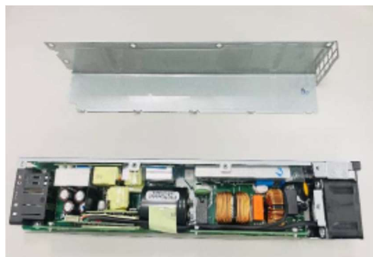
Figure54 Use tool#1 to unscrew six screws to loosen PCBA from bottom chassis
