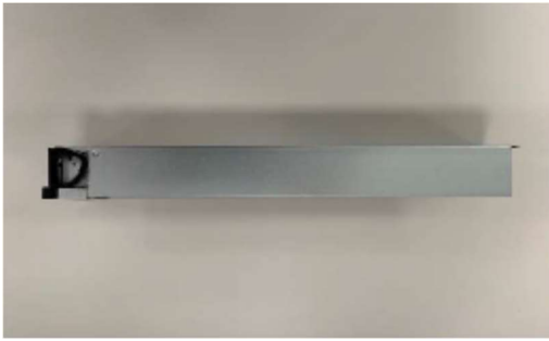
Figure63 Slide handle-released module away from bottom chassis.
