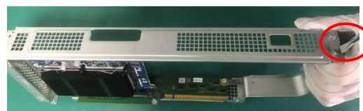
Figure12 Use to PH1 screwdriver to uninstall the screws of extender single slot.
