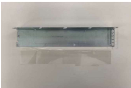
Figure53 Remove the Mylar from top cover by hand-pulling
