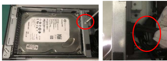
Figure20 Remove to the cable from the internal HDD cage.
