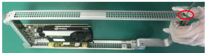
Figure4 Use to PH1 screwdriver to uninstall the screws.
