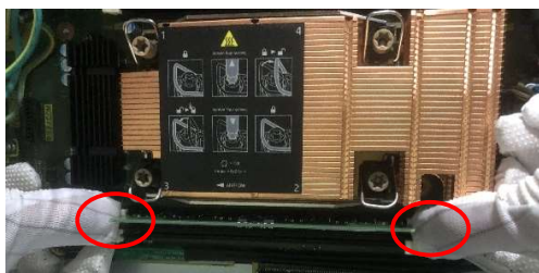
Figure7 Remove the memory from MB.
