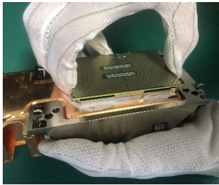
Figure19 Remove to the CPU from the CPU heatsink.
