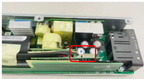
Figure57 Remove the Mylar from bottom chassis by hand-pulling.
