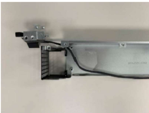
Figure63 Slide handle-released module away from bottom chassis.
