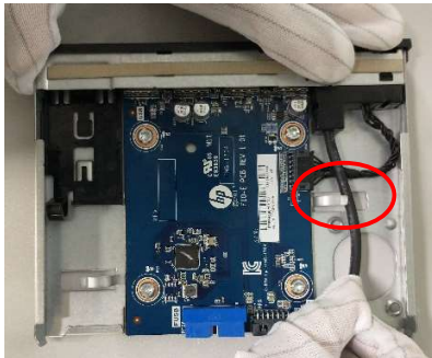
Figure33 Release the front panel mount cable from clip
