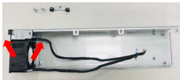
Figure59 Remove fan from the bottom chassis by hand-pulling upwardly
