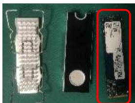
Figure11 Remove the extender single slot from M/B.
