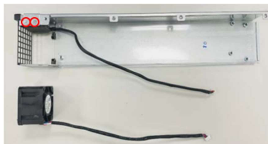
Figure60 Use tool#2 to unscrew two screws to loosen handle-released module from bottom chassis.
