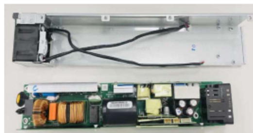
Figure58 Use tool#1 to unscrew four screws to loosen fan from bottom chassis
