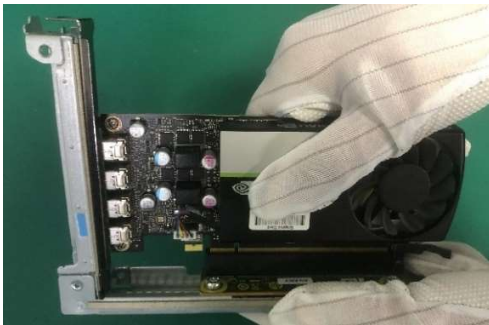
Figure5 Press the graphic card's latch and remove it.
