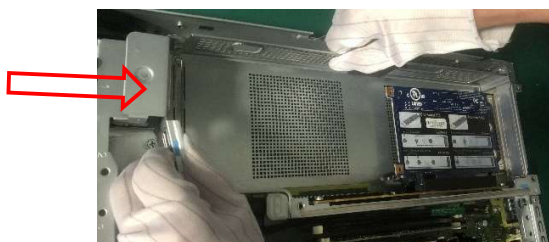
Figure11 Remove the extender single slot from M/B.
