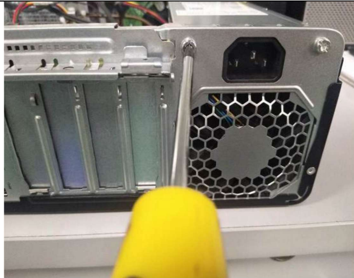
Step27 Remove the Power supply from chassis
