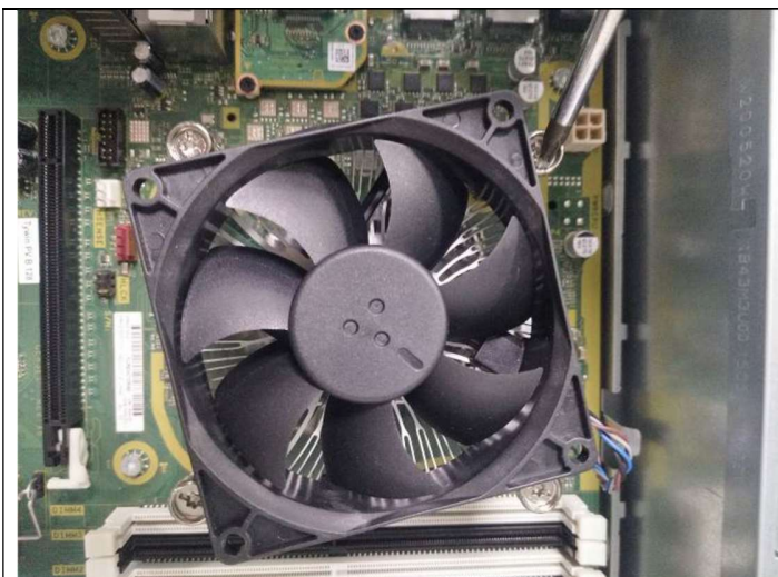
Step15 Separate the fan from CPU heat sink
