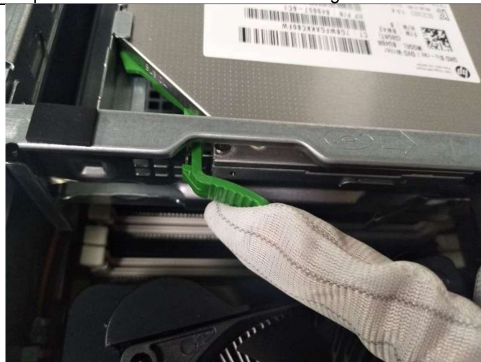
Step5 Remove Front Bezel from chassis
