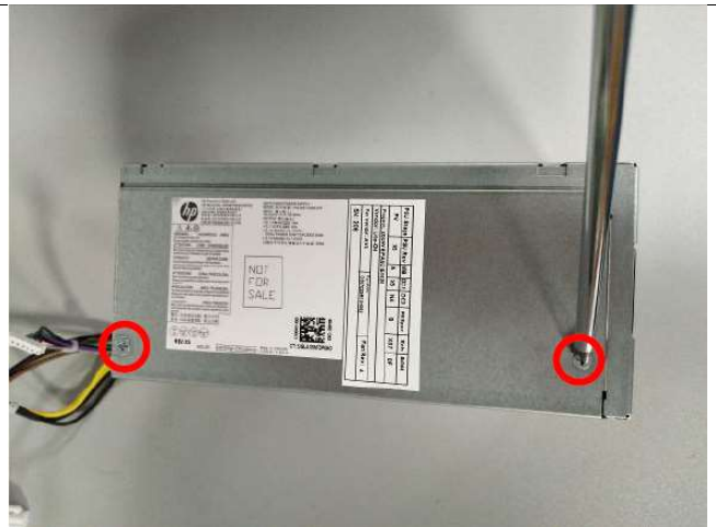
Step30 Use PH1 screw driver to remove FG screw
