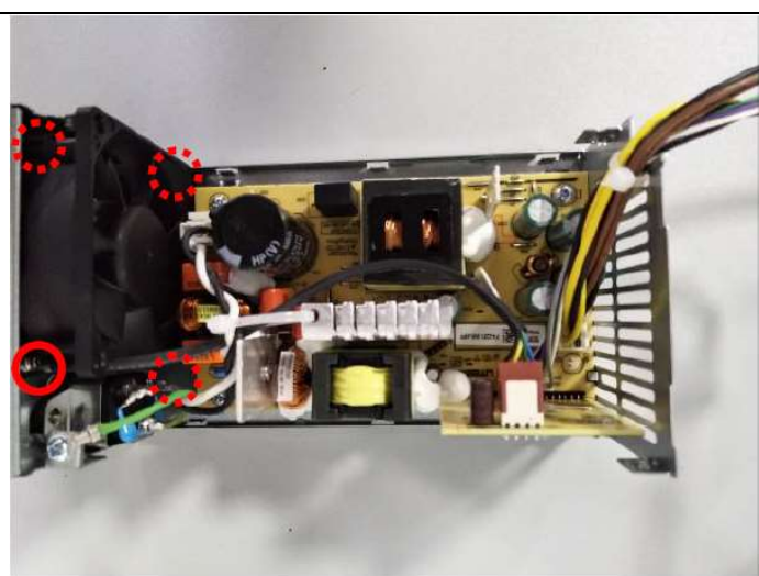
Step33 Loose screws and remove PSU fan
