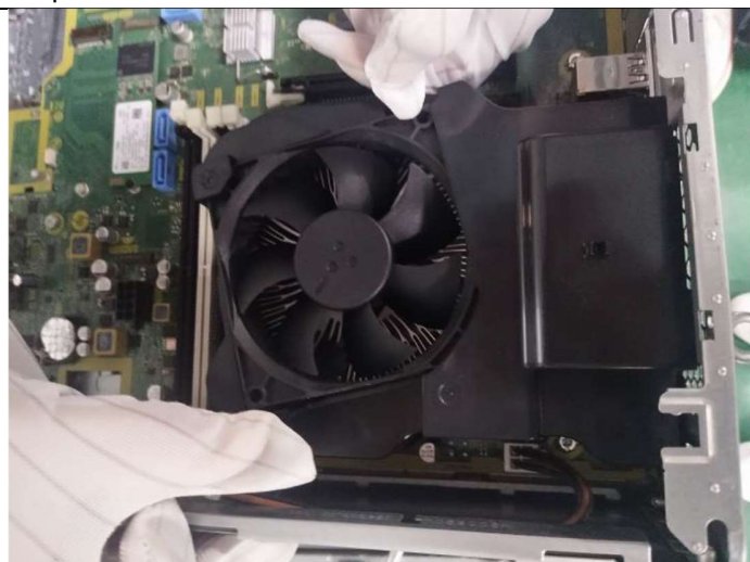
Step13 Use T-15 screw driver to loose the cooler screws and remove cooler from MB
