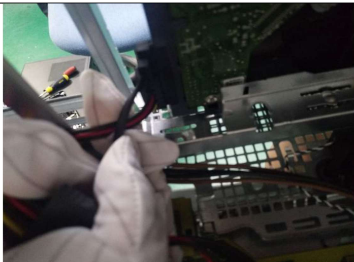
Step8 Use T-15 screw driver to loose the screws of HDD
