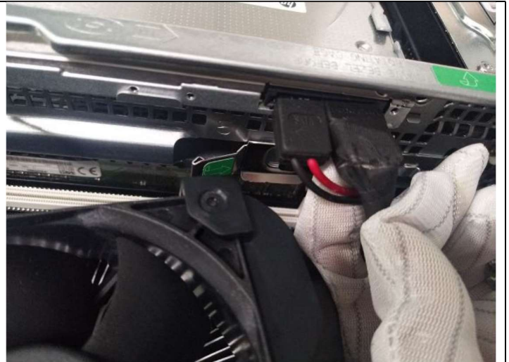
Step4 Remove the ODD from ODD cage
