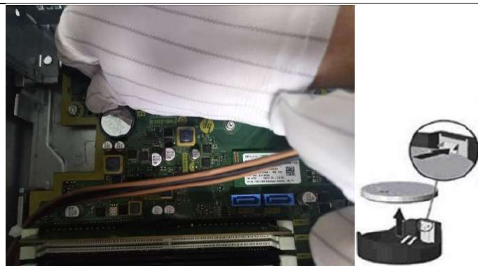
Step21 Remove the battery from the system board
