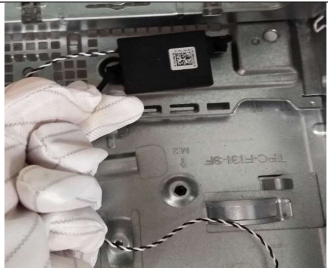
Step26 Press the Power supply's latch on chassis
