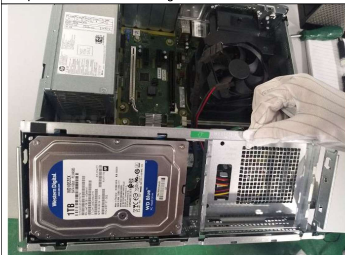
Step9 Remove HDD from HDD cage
