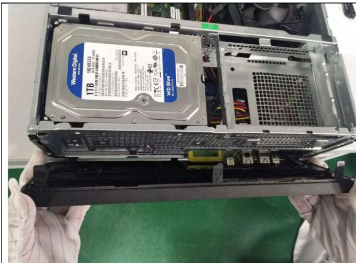
Step7 Remove the drive cage from Chassis
