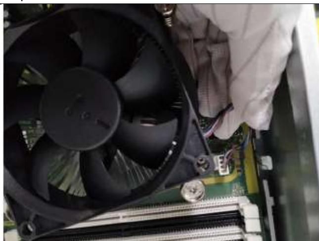
Step12 Disconnect Cooler Fan cable from MB
