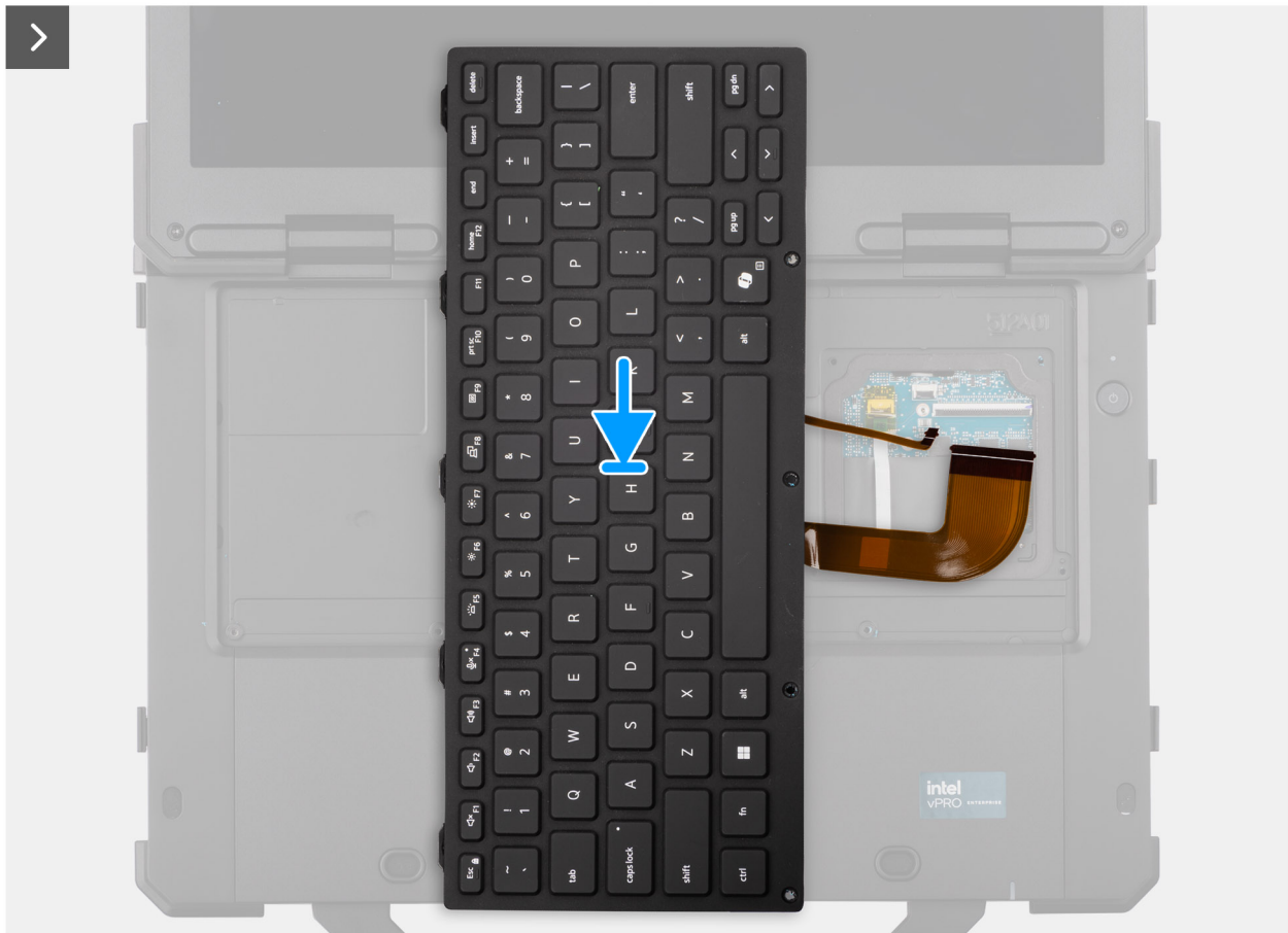
Figure 33. Installing the keyboard (rubberized)
