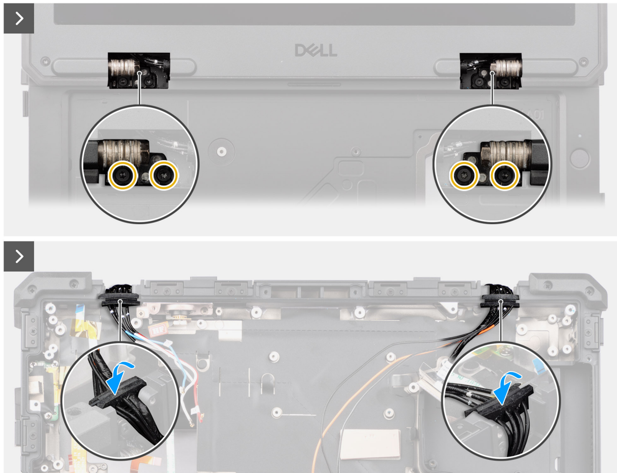
Figure 122. Installing the display assembly
