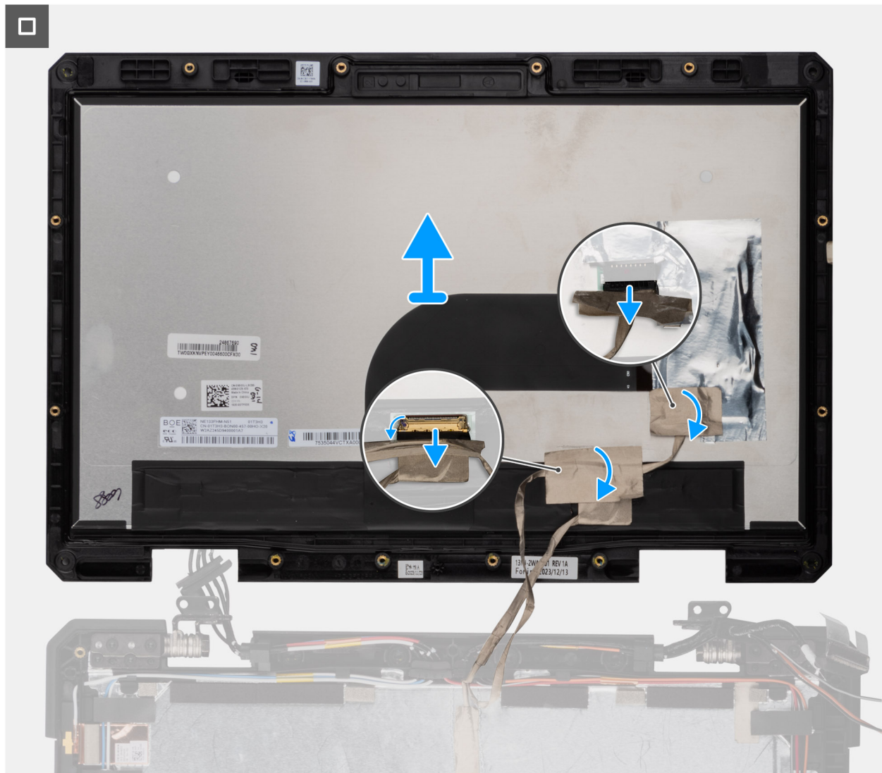
Figure 125. Removing the display-panel assembly
