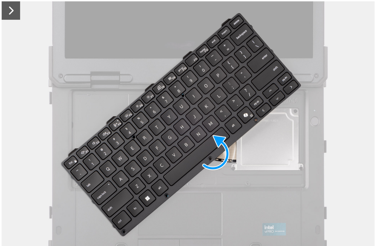
Figure 23. Removing the keyboard (standard)
