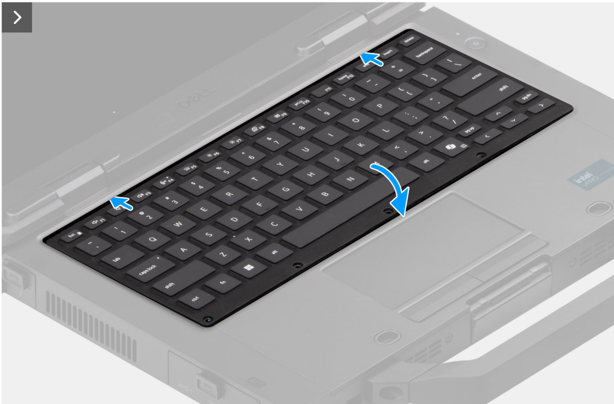
Figure 35. Installing the keyboard (rubberized)
