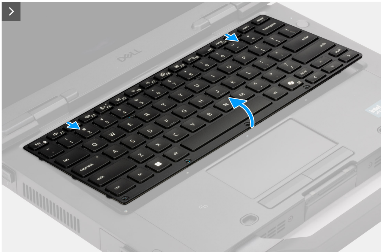
Figure 22. Removing the keyboard (standard)
