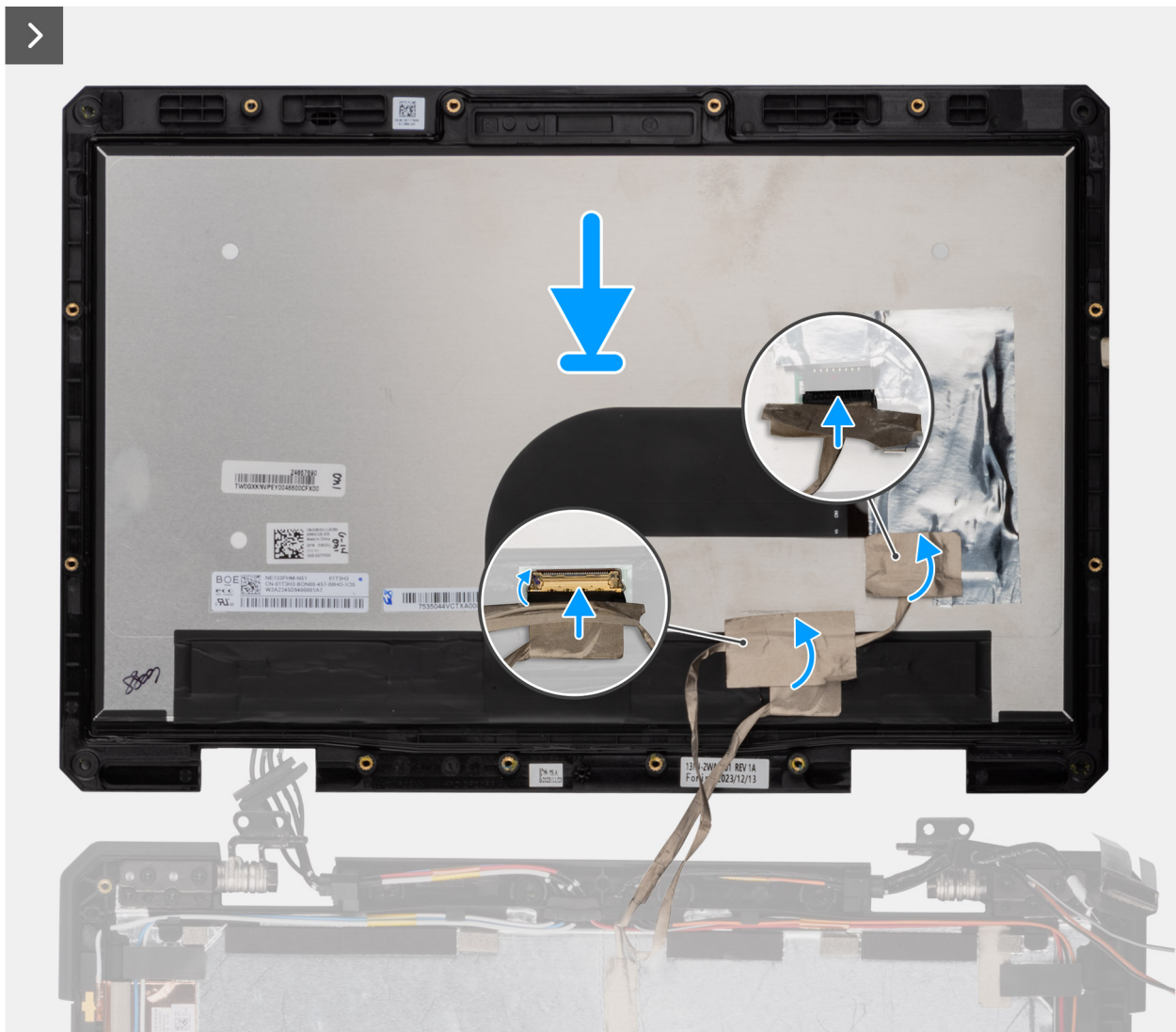
Figure 126. Installing the display-panel assembly
