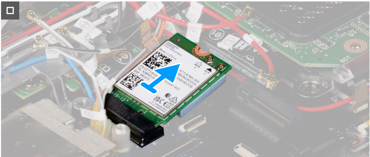
Figure 74. Removing the WLAN card
