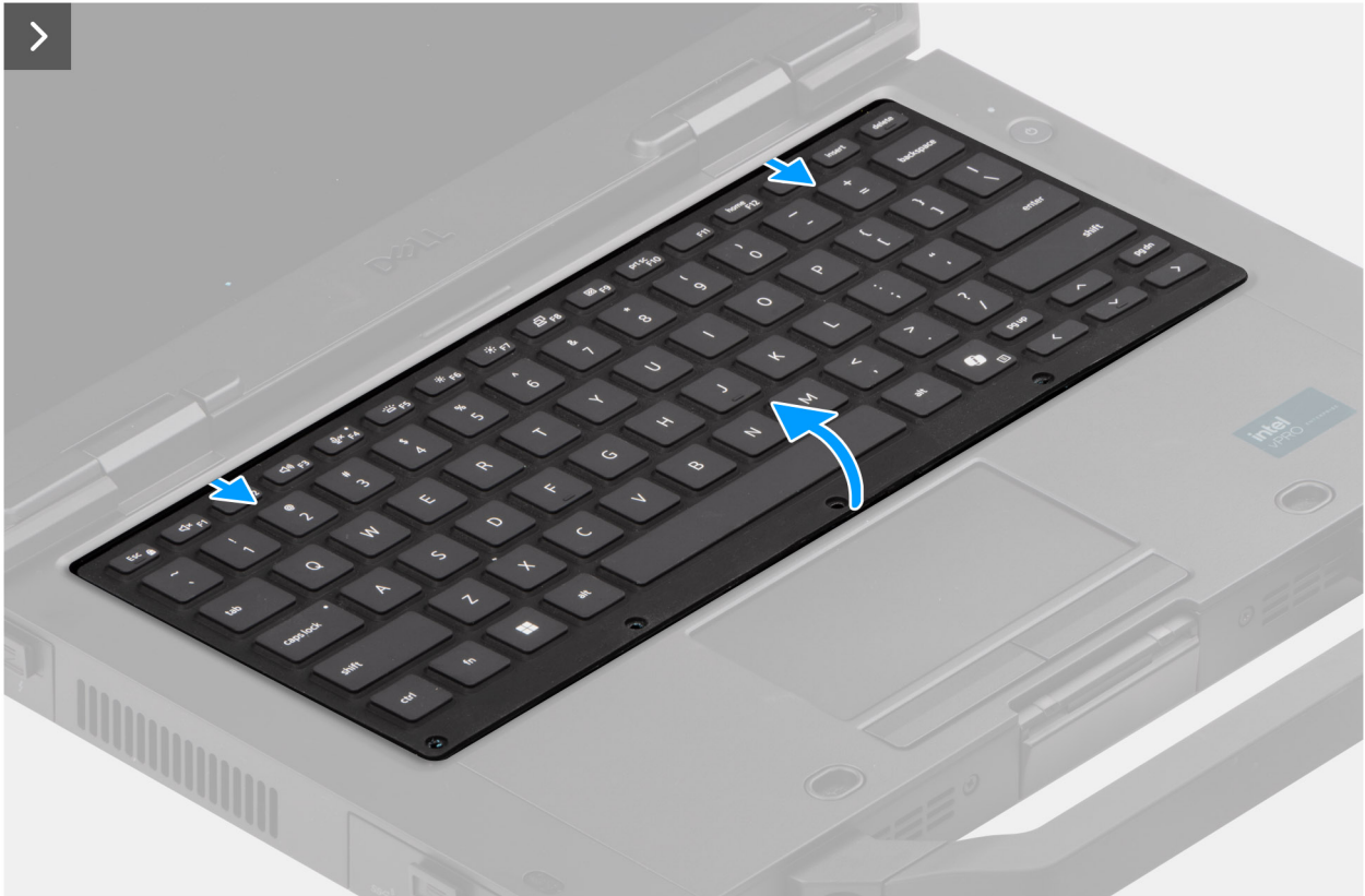
Figure 30. Removing the keyboard (rubberized)
