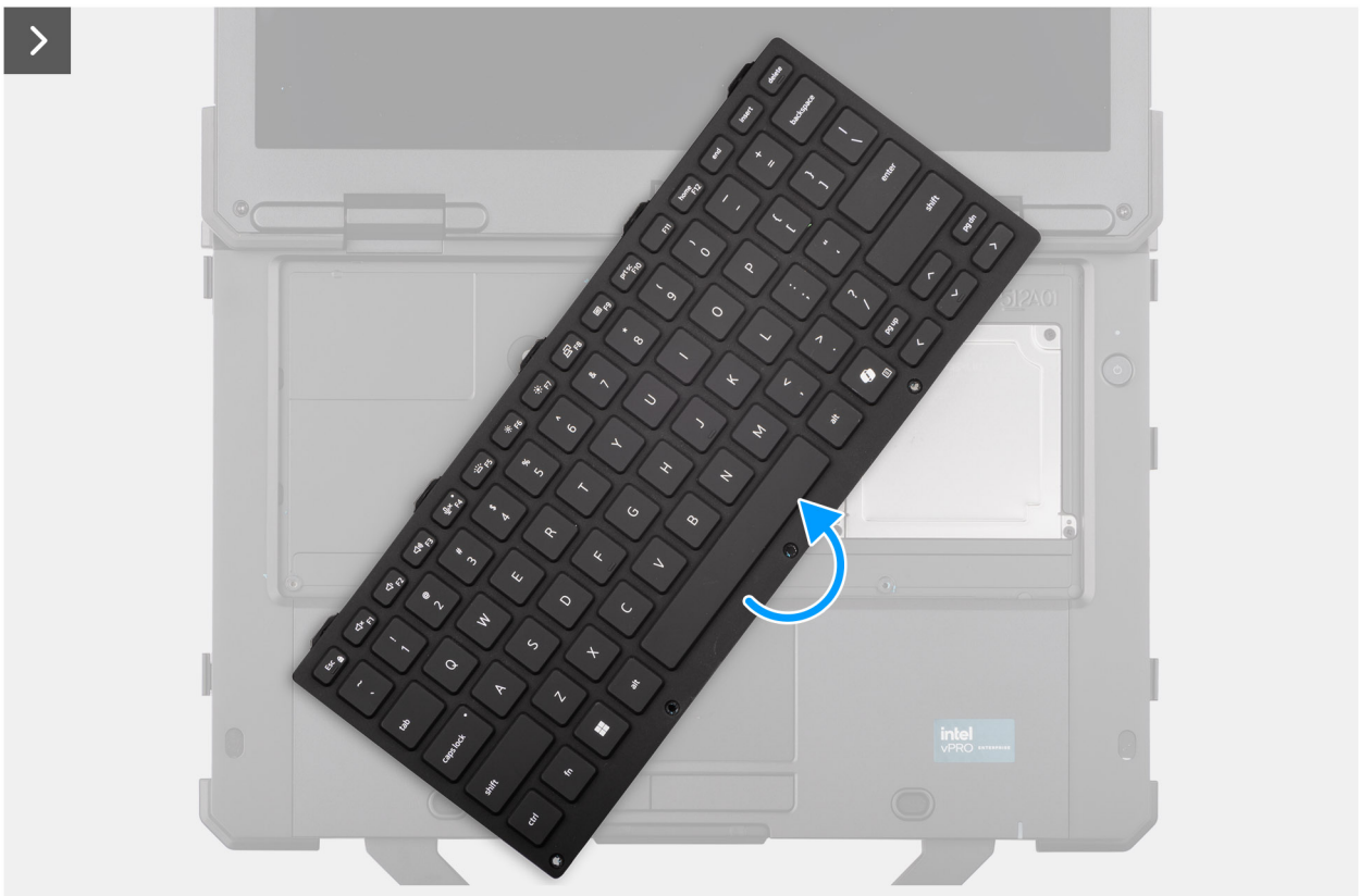
Figure 31. Removing the keyboard (rubberized)
