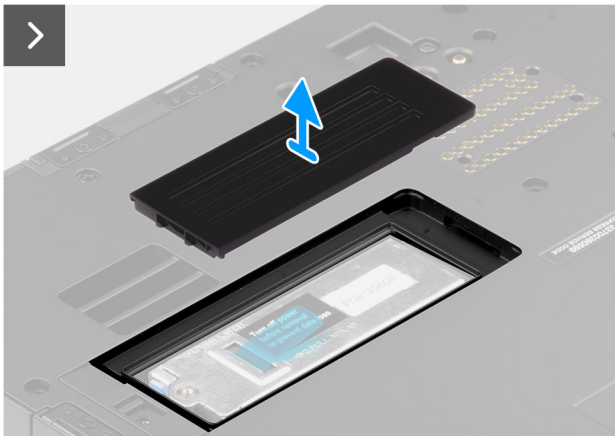
Figure 37. Removing the solid state drive carrier
