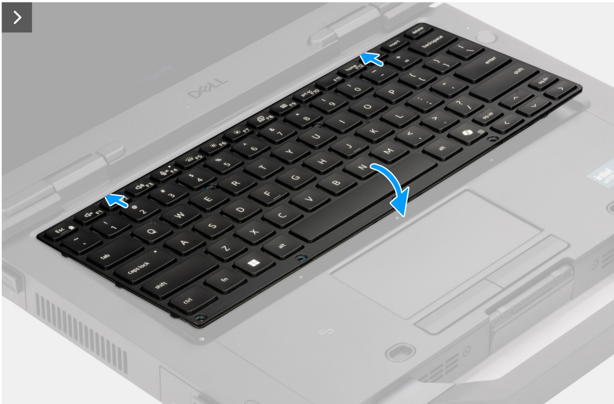
Figure 27. Installing the keyboard (standard)
