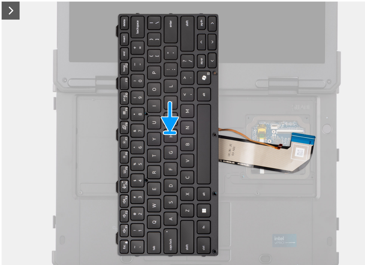
Figure 25. Installing the keyboard (standard)
