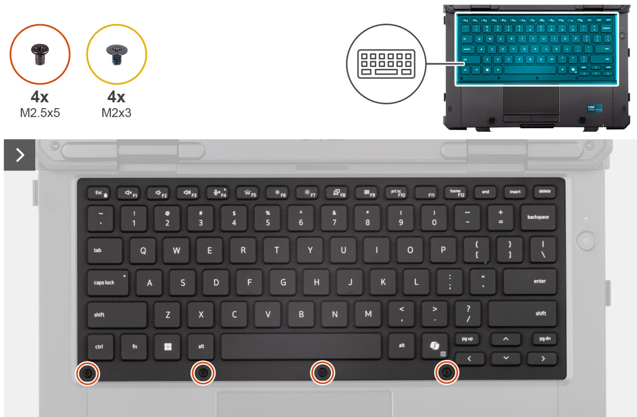
Figure 29. Removing the keyboard (rubberized)
