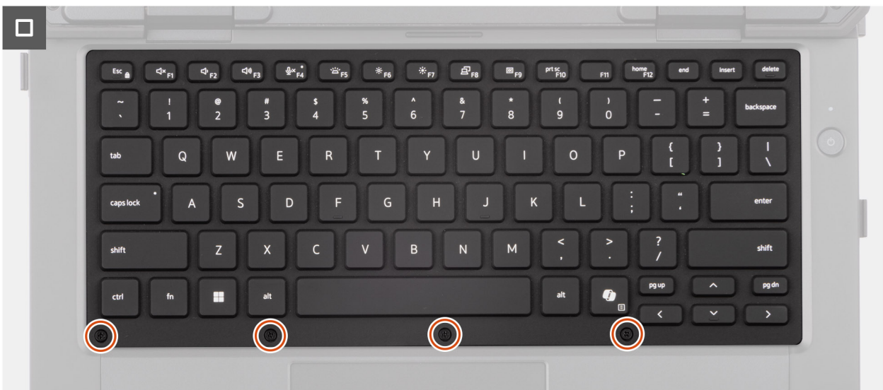
Figure 36. Installing the keyboard (rubberized)
