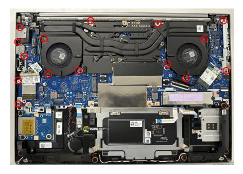
3.24 Release below cable: Speaker cable, Finger Printer cable, backlight cable, TP cable, SD card cable, SIM card cable, KB Cable, EDP cable, WWAN antenna cable, WLAN antenna cable. And Disassemble Type-C BKT, RJ-45. Final step release main board
