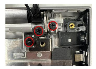
3.26 Set Hinge UP to 90 degree and release hinge up
