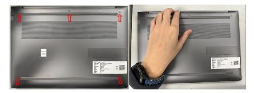
3.22 Use screwdriver to release battery screw 4 PCS and release Battery
