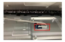
**S5** Tear off a tape from CTRL BD FFC and Rear Cover
