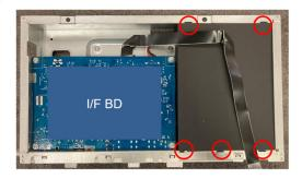
**S20** Unlock 8 PCBA screws to disassemble I/F BD, SPS BD from Main SHD
