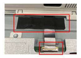
S16 Unlock 13 MF screws and 2 MF screws (M3\*9) to disassemble Middle Frame
