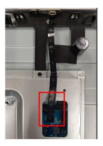
**S8** Disassemble "SENSOR BD" from Middle Frame
