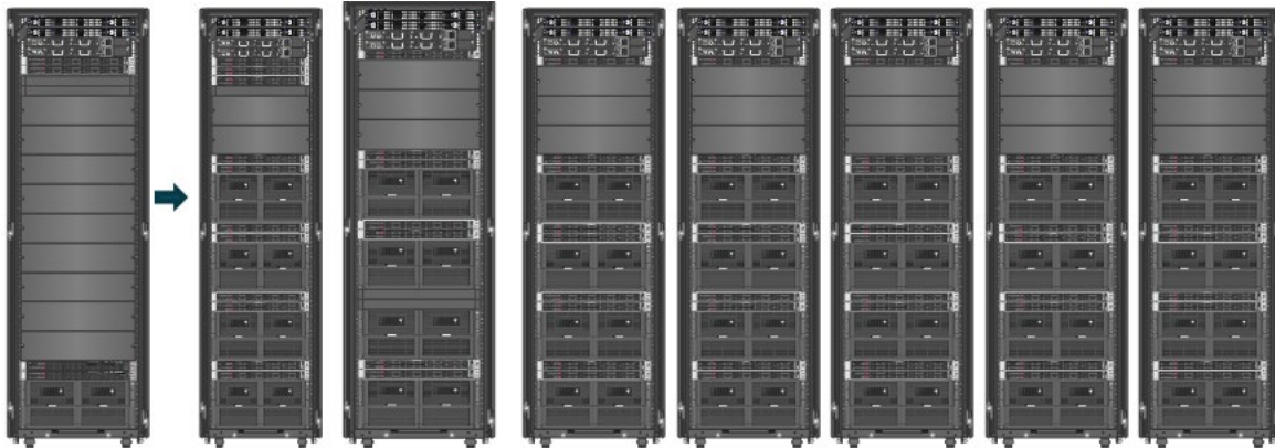
FIGURE 9. The HPE ConvergedSystem 300 for Microsoft Analytics Platform solution scales from a “Quarter Rack” up to seven racks
