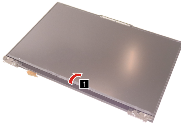
Figure 33. Remove the hinge cover
