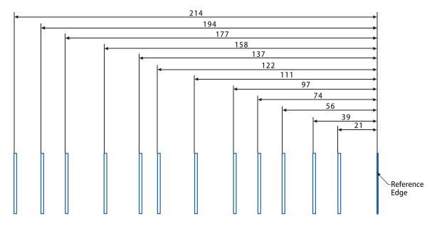
Rib pattern for Lexmark B2865, M5255, M5265, M5270, MB2770, MS725, MS821, MS822, MS823, MS824, MS825, MS826, MX721, MX722, MX725, MX822, MX824, MX826, XM5365, XM5370, XM7355, XM7365, XM7370
