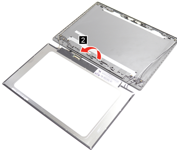
Figure 33. Rotate the LCD panel
