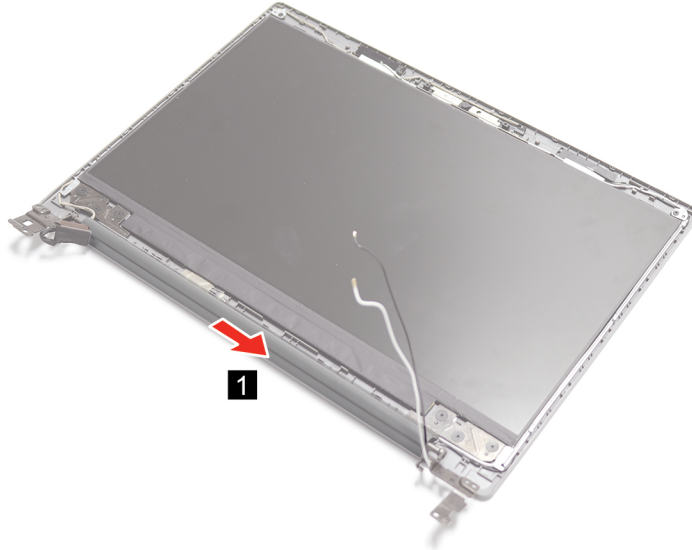
Figure 30. Remove the hinge cover
