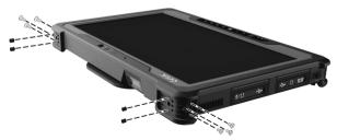
2. Noting the orientation (stylus slot in the front), attach the handle to A140.
