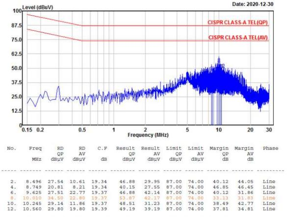
Remarks: C.F (Correction Factor) = Insertion loss + Cable loss + Pulse Limiter
