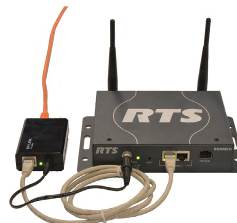
Figure 3. How to connect the PoE adapter
