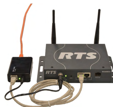
Figure 3. How to connect the PoE adapter
