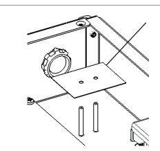
10. Slide the *Terminal Block Insulator* down over the two threaded studs.
