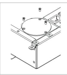
9. Install the *L14 Close-off Plate*, and secure it in place using the flat head screws provided.
