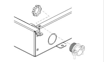
4. Install the *¾-inch strain relief cable clamp*, and fasten it into place using the locknut provided.
