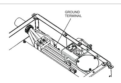
15. Remove the nut loosed in step 7 from the ground terminal on the chassis, slide the *ground wire ring lug* over the ground terminal, and secure it in place with the nut, torque setting 11in lbs ~ 13 in lbs.
