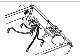
16. Attach the wires from the *TBA* to the *PCB Reference Points*, listed in Table 1. These points differ slightly for each model, as shown in the table.
