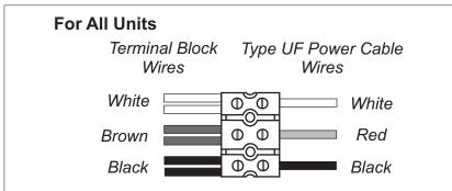
13. Thread the *Type UF Power Cable* through the *Strain Relief Cable Clamp* (shown in *step* 4), and insert the white, red and black wires into the *TBA* shown above. Tighten the screws to secure the wires in place, torque setting 10 in lbs ~ 16 in lbs.
