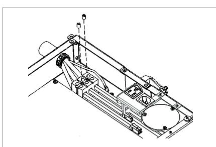
14. Slide the *TBA* down over the two (2) threaded studs, shown in Step 10, and install the two (2) *slotted nuts*, as shown above.
