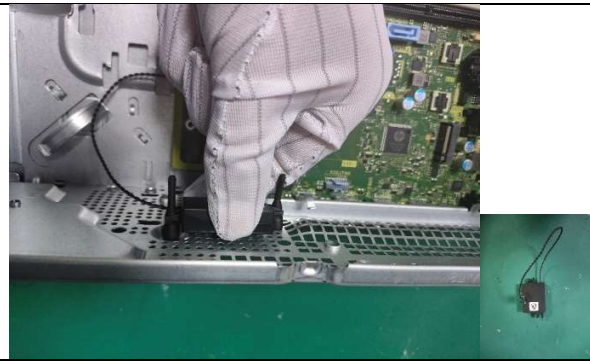
Step20 Remove the Motherboard from Chassis.
