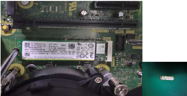
SSD PCA area surface is greater than 10 sq cm.
