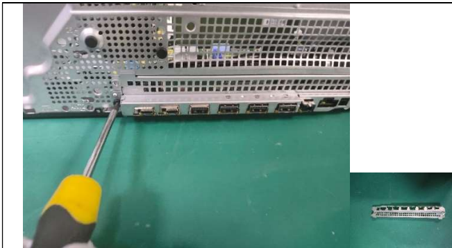
Step11 Loose the Screws from SSD and remove it.
