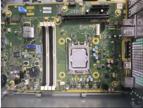
Step21 Remove the CPU from the Motherboard.
