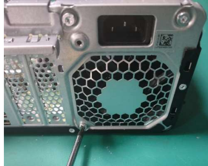
Step16 Press the holder and remove the PSU from the chassis.
