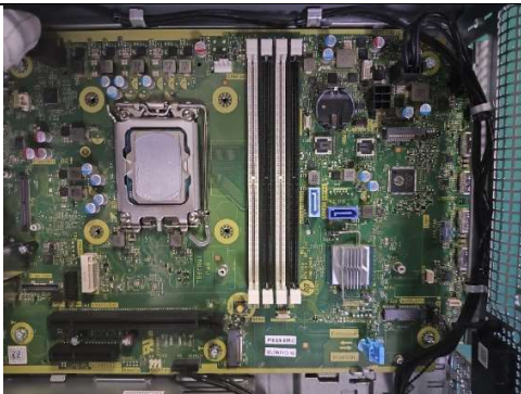
Step17 Remove the speaker power cord from the motherboard.
