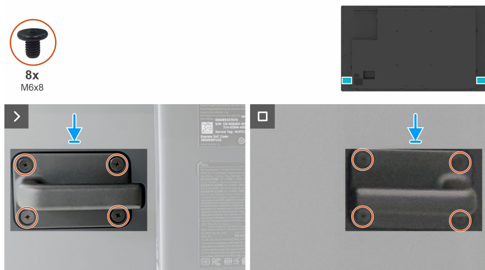
Figure 25. Installing the handles
