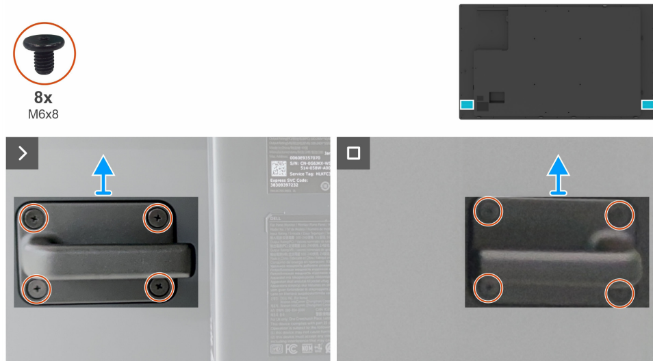
Figure 24. Removing the handles
