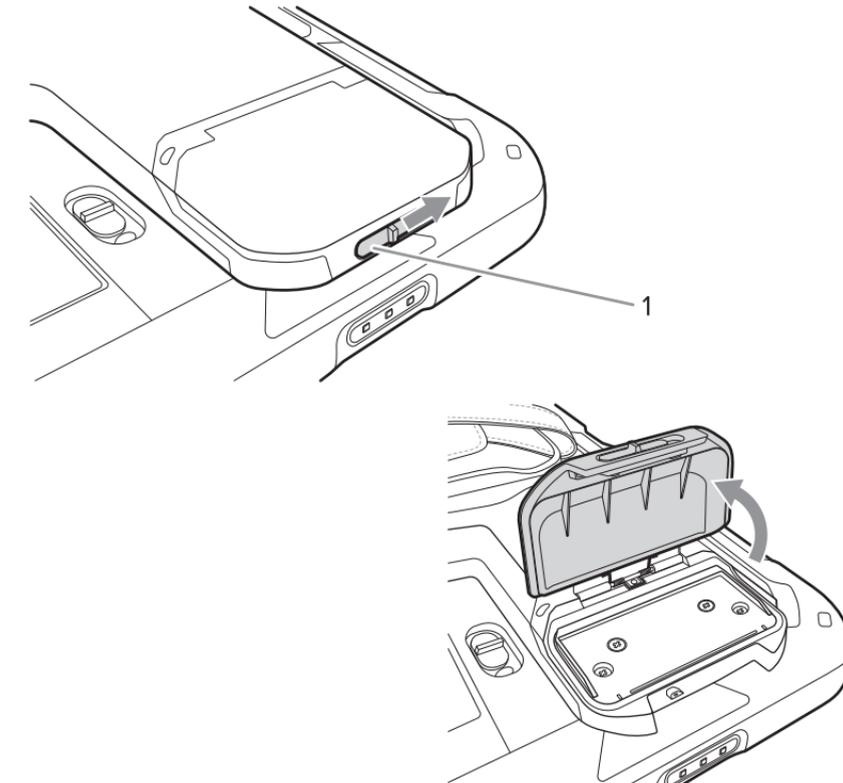
Insert the card (chip facing down) into the card slot (1).
