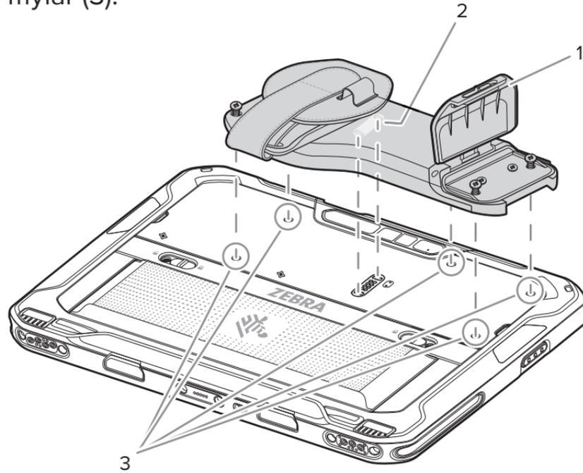
4. Secure the Reader to the tablet using five captive screws. Torque to 4.5 kgf-cm (3.9 lbf-in.).
