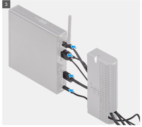
Align the cable cover retaining hooks into the slots on the system chassis.
