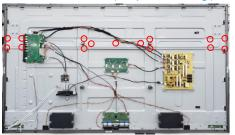
S12 Disconnect the touch cable and FFC cables. Use a screwdriver to remove 24pcs(16+8) screws
