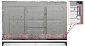
Use a screwdriver to remove18pcs screws for unlocking the two VESA brackets with back bracket.(Torque: 5±0.5kgf)
