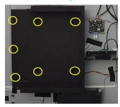
S3 Paste 1pcs for fixing the cable as the picture below shown. Remove 16pcs acetate tapes(size: 80mm) and 1pcs acetate tapes(size: 60mm) for unfixing the cables as the picture below shown.
