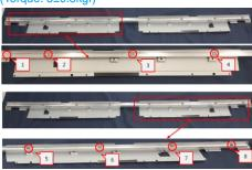
Tear off 16pcs acetate tapes, then use a screwdriver to remove 17pcs screws for unlocking the bottom-middle bezel.(Torque: 3.5±0.3kgf)
