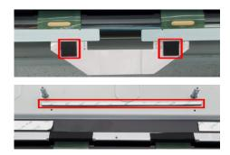
Turn over the panel module with the bracket for screen faced up. Use a thin film(such as Prism film) to disassemble the O/C with glass carefully, then remove the O/C with glass and put then on a protective cushion.
