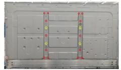
Tear off the papers of the tapes on the L/B heat sink, then assemble the L/B heat sink with back bracket. Use a screwdriver to tighten 33(25+8)pcs screws for locking the L/B heat sink with the back bracket. Paste 2pcs rubber on the specific positions of the back bracket as the below picture. (Torque: 5±0.5kgf)
