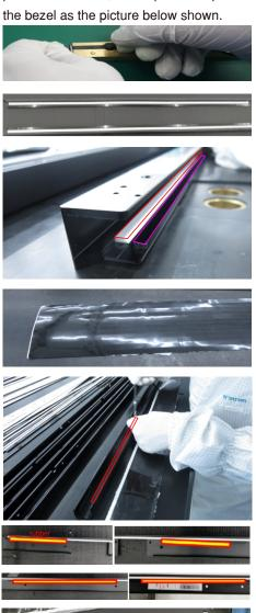
Take 1pcs light pipe, and then use a screwdriver to lock 2pcs screws for locking the light pipe with front bezel. Take 1pcs IR board and 1pcs IR holder and 1pcs shading tape, then assemble the IR board with IR holder, then use a screwdriver to lock 2pcs screws for locking the IR holder with front bezel, then assemble 1pcs IR board cover to bottom-side bezel.
