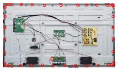
Use a screwdriver to remove 2pcs screws for unlocking the key board and the holder with strip. (Torque: 2±0.3kgf)
