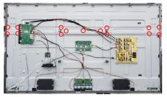
Assemble 4pcs front bezels(top, left, right, bottom) with the assembled unit, then use a screwdriver to tighten S26 38pcs screws for locking the front bezels with the assembled unit.(Torque: 3±0.3kgf)
