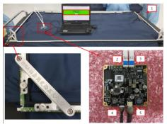
Disconnect the bottom ED holder away from the left S12 and right ED holders, then replace the bottom ED holder with a fixture Jip as the picture below shown.
