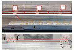
Assemble 2pcs fixture rubber on the side of the back bracket, then place 1pcs Reflector film into the back bracket. Make sure the gap between light and Reflector >1.2mm.
