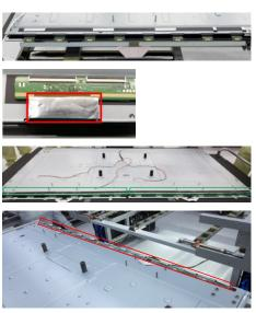
Take 1pcs top front bezel, 1pcs left front bezel, 1pcs right front bezel, 1pcs bottom front bezel, 4pcs filter films, 6pcs reflector (long 4pcs and short 2pcs), then paste the reflector, filter tapes and 4pcs rubbers on the bezel as the picture below shown.
