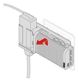
Remove the power cord from the power adapter. See "Power adapter and power cord" on page 34.
