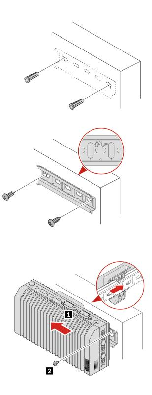
The replacement steps also apply to the computer with an IO expansion box installed. See "IO expansion box" on page 35.
