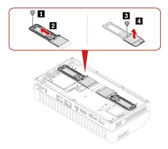
**Note:** After installing the new M.2 solid-state drive, ensure that you attach the new thermal pad to the new M.2 solid-state drive.
