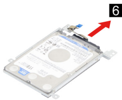
Figure 44. Remove the HDD cable
