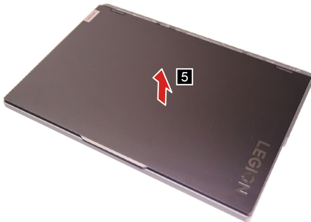
Figure 32. Remove the LCD unit
