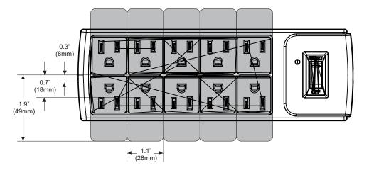
FTT699: 6 x Large Adapters on 6 Outlet Power Bar FTT1112: 10 x Large Adapters on 10-Outlet Power Bar
