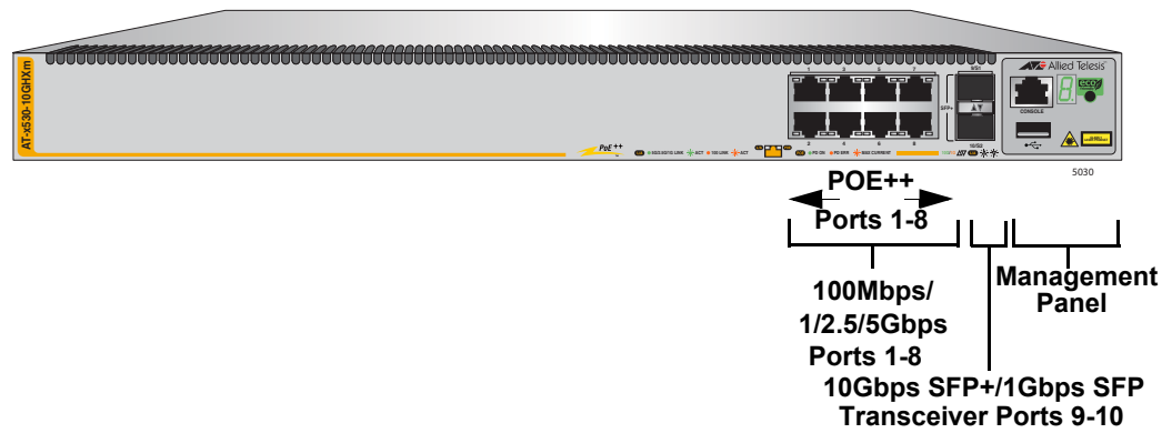
Figure 1. Front Panel of the x530-10GHXm Switch
