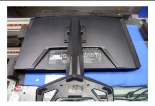
Remove the screw \* 4pcs Tool : Screwdriver #2
