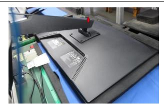
Wedge your fingers between the rear cover and the middle bezel on the corners of the top side of the monitor to release the rear cover Tool: Gloves
