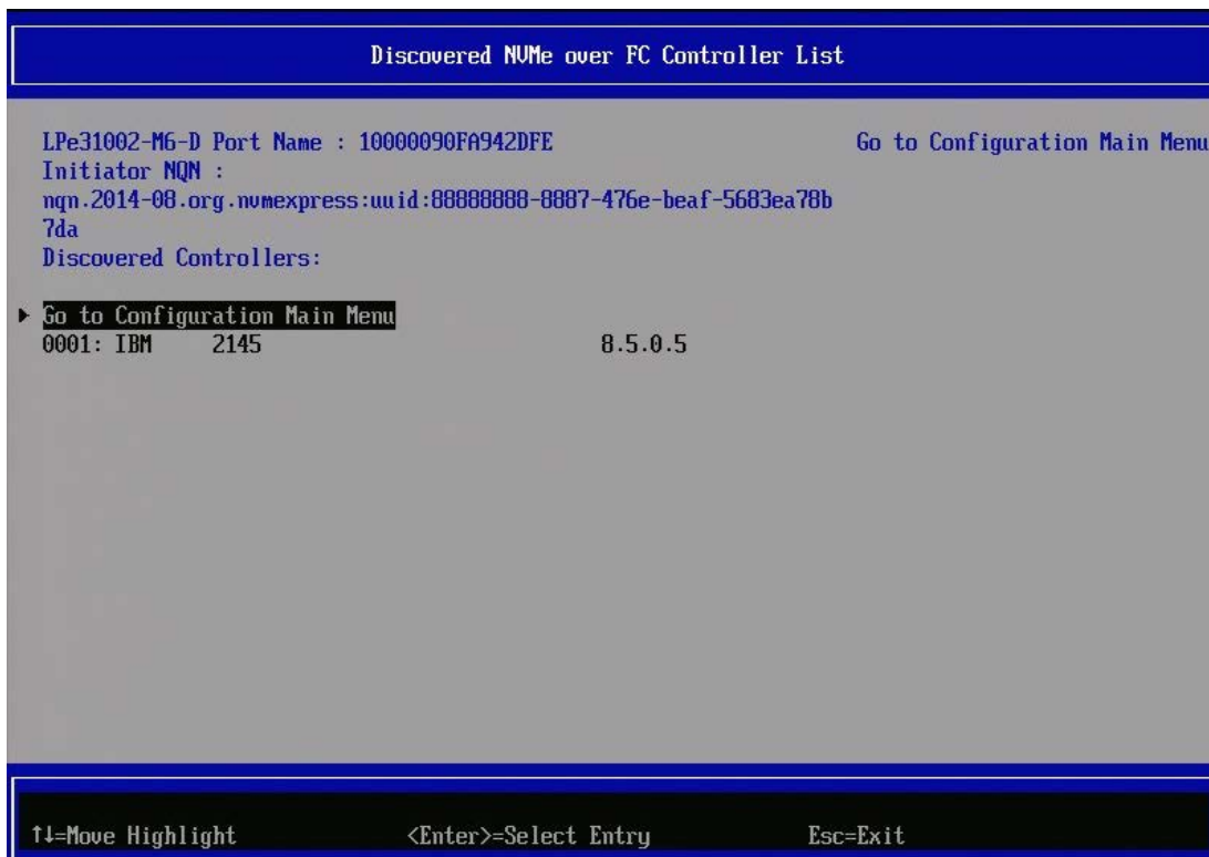
Figure 33: Discovered NVMe over FC Controller List Window
