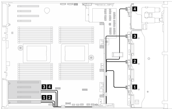
Figure 20. SAS/SATA cable routing to bottom PCIe zone
