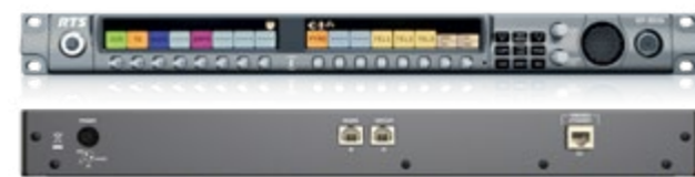
KP-3016 ONE RACK UNIT KEYBOARD, 16 OPERATION KEYS WITH ANALOG AND IP (OMNEO/DANTE OR RVON) MATRIX INTERFACE
