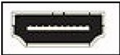
Identifying an HDMI 19-pin port.
