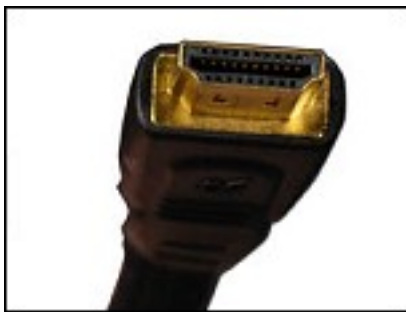
Identifying an HDMI 19-pin port.
