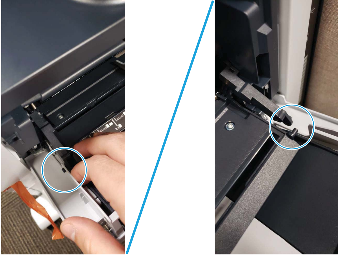
Figure A-5 Release lift plate and support tray assembly
