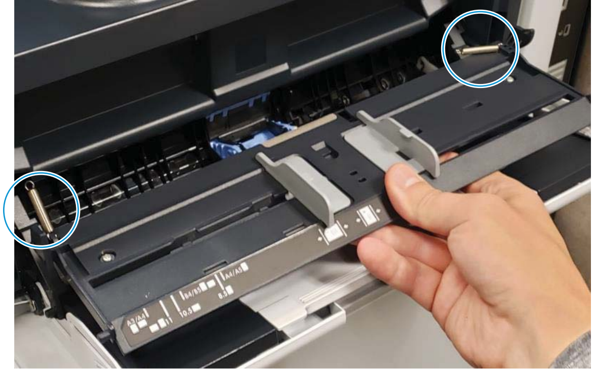
Figure A-10 Install the retained springs
