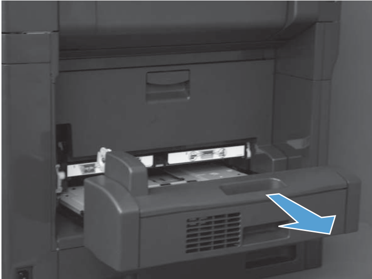
Figure 1-43 Remove the duplexer (1 of 2)
