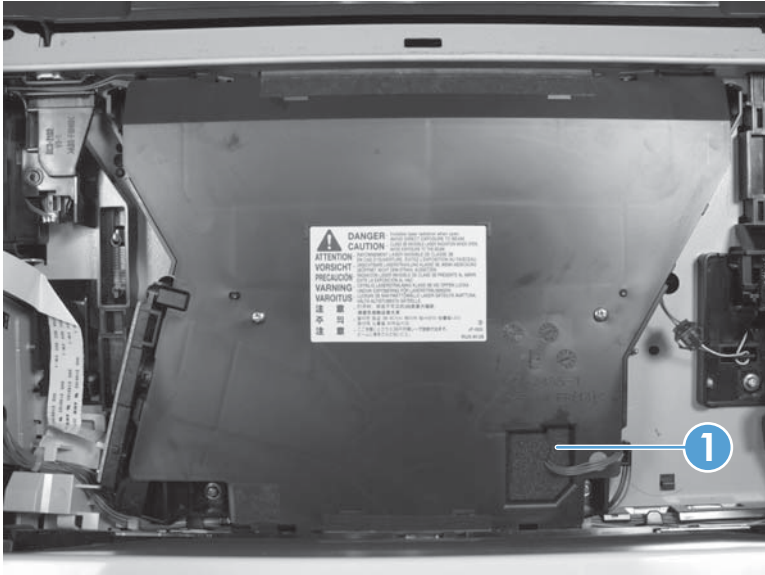
Figure 1-67 Remove the laser scanner (1 of 3)
