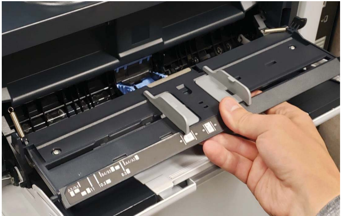
Figure A-11 Install the lift plate and support tray assembly
