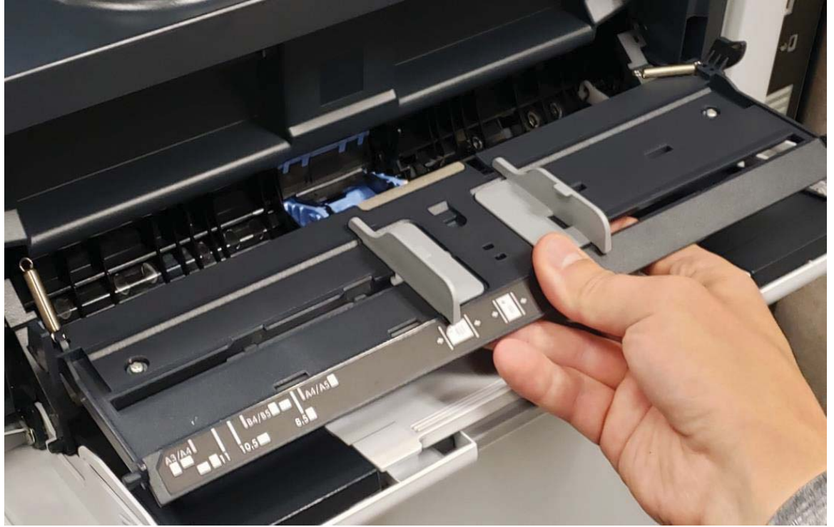
Figure A-6 Remove the lift plate and support tray assembly
