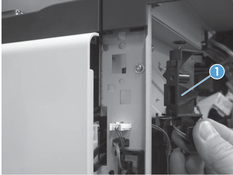
Figure 1-112 Remove the cartridge door interlock switch (3 of 4)
