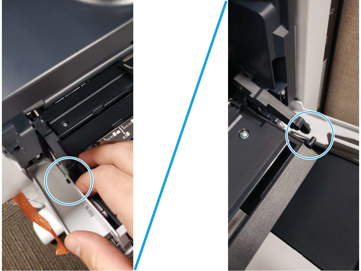
Figure A-12 Engage the lift plate and support tray assembly and door
