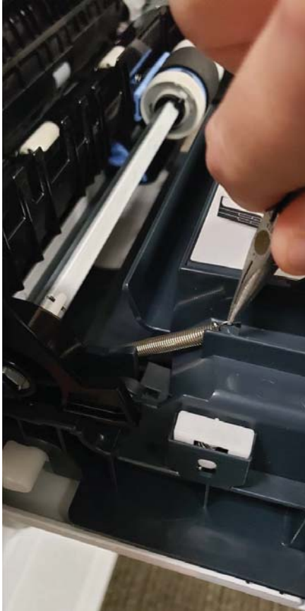
Figure A-3 Release the springs
