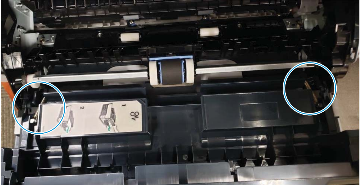
Figure A-13 Reattach the springs
