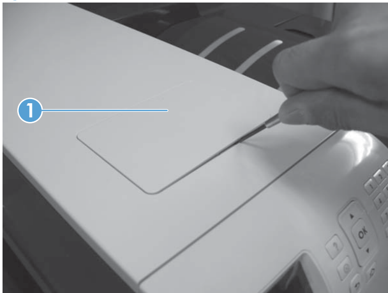
Figure 1-27 Remove the top cover (1 of 2)
