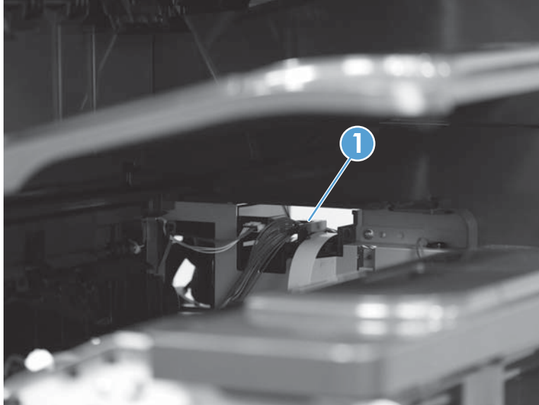
Figure 1-49 Remove the paper delivery assembly (1 of 2)
