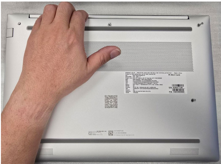
And disassemble base cover from hinge side
