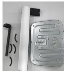
7.2 Remove the base, rubber and cable holder
