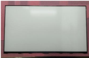
8.2 Uncover the plastic frame to separate the OC
