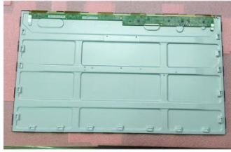
8.2 Uncover the PCBA to separate it from the backplane
