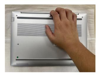
3.22 Rotate hook to unlock battery and release battery cable then release battery
