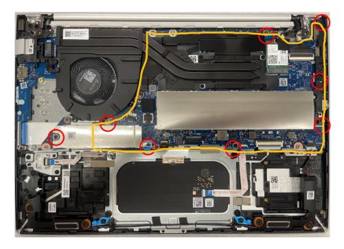
3.24 Release below cable: Speaker cable, Finger Printer cable, backlight cable, KB cable, TP cable, IO board cable, EDP cable, Fan cable, WWAN antenna cable, WLAN antenna cable. And Disassemble IO frame, RJ-45 frame. Final step release main board
