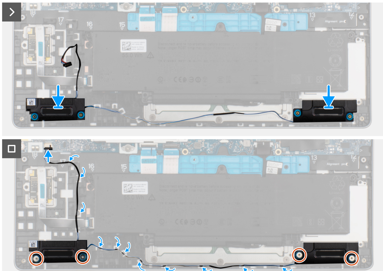
Figure 35. Installing the speakers
