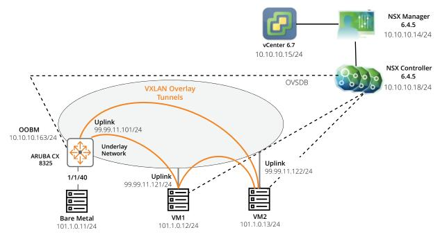
Figure 1: Network Topology for VMware NXS-V and Aruba CX 8235 Integration
