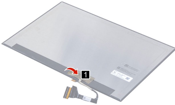
Figure 45. Peel off the tape
