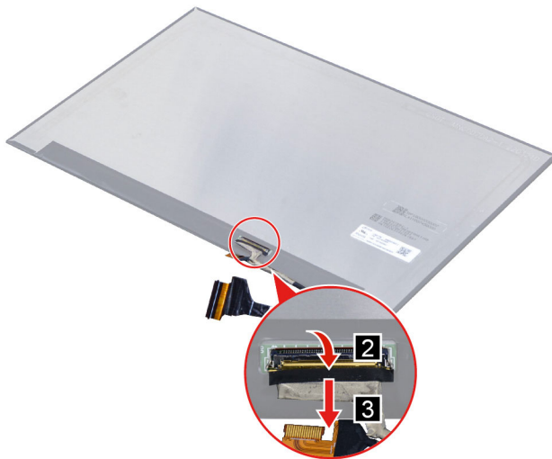
Figure 46. Remove the EDP cable
