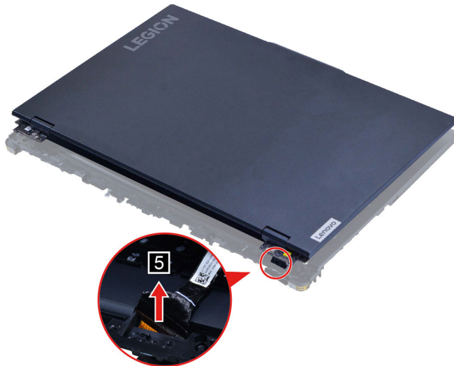
Figure 35. Take out the EDP cable and remove the LCD module
