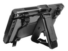
**NOTE:** When closing the hand grip, be sure to fold up the flexible band properly. Keep the folded band inside the hand grip in a flat and smooth condition.
