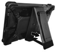
**NOTE:** When closing the hand grip, be sure to fold up the flexible band properly. Keep the folded band inside the hand grip in a flat and smooth condition.
