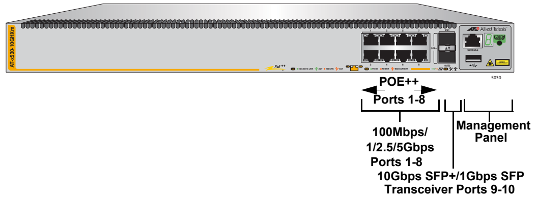
Figure 1. Front Panel of the x530-10GHXm Switch
