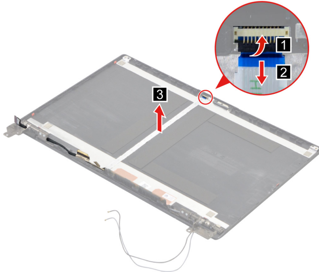
Figure 38. Disconnect the EDP cable from the camera board and then remove the EDP cable
