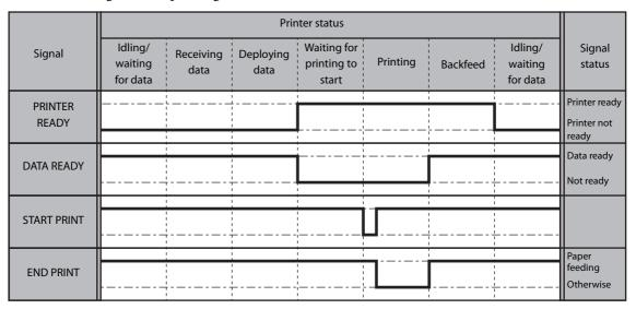
The pin 18 end print signal is indicated when Mode 1 (= the printer feeds paper during Low) is set, and when the setting value for the "backfeed operation time settings" menu is "backfeed after label is issued".
