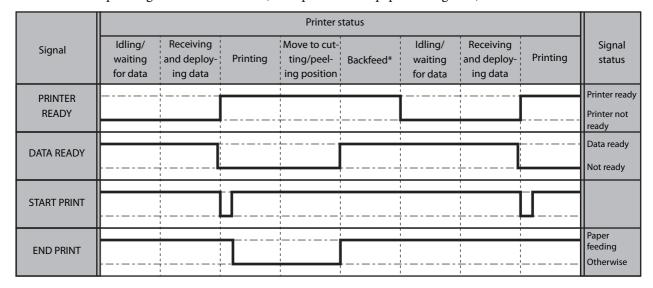
\* After the label moves to the cutting/peeling position, it is held for 300 ms (initial setting). When this time has elapsed, a backfeed operation is performed. The initial setting can be changed.
