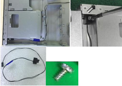
Step55 Remove LED cable assembly by screwdriver T15
