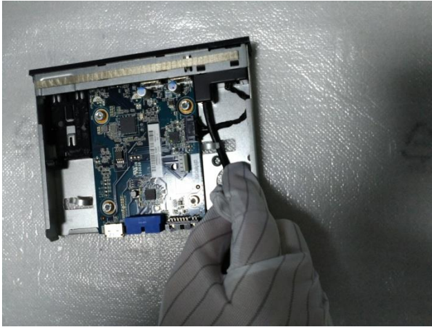
Figure33 Press the 4 latch and remove the front UI/Audio ASSY cable from FIO module
