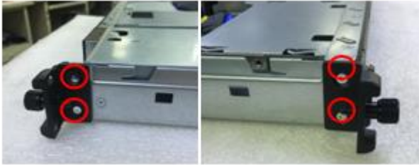
Step39 Remove rack hand brackets by screwdriver T15
