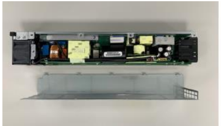
Step60 Remove top cover from bottom chassis
