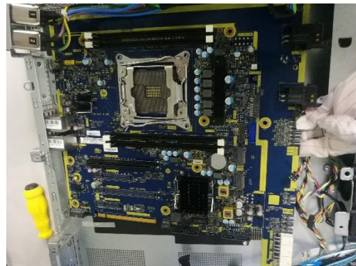
Step23 Use PH1 screwdriver to loose the screws and remove the led flatiron
