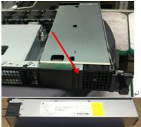
Step59 Slide top cover to unhook bottom chassis before top cover removal
