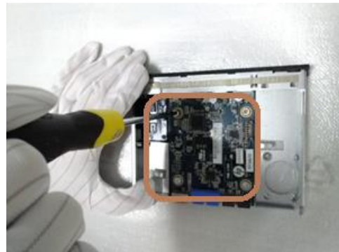
Figure34 Loose the 4 screws of PCA and remove the PCA from FIO module. See below PCA area>10 sq cm.
