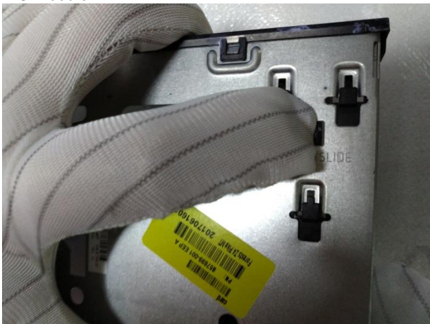
Figure35 Press the latch and remove the SD card holder from FIO module
