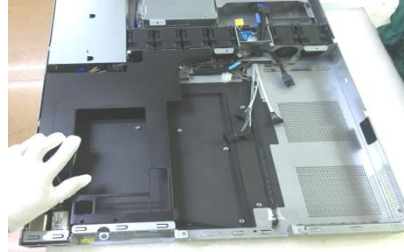
Step38 Remove air duct
