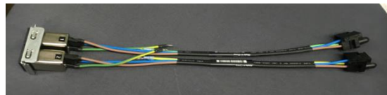
Step42 Remove metal bracket of internal AC cable
