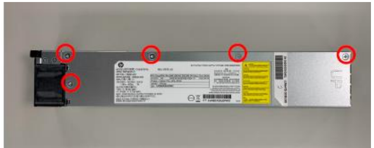
Step58 USE PH1 to unscrew five screws to loosen top cover
