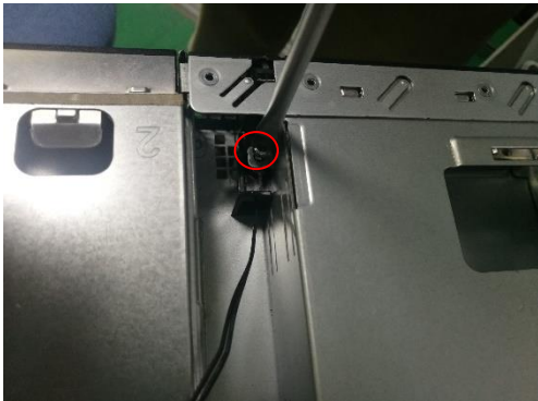
Step23 Use PH1 screwdriver to loose the screws and remove the led flatiron
