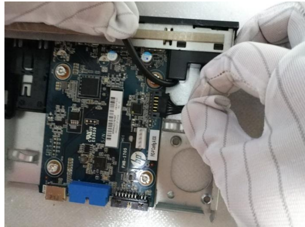
Figure34 Loose the 4 screws of PCA and remove the PCA from FIO module. See below PCA area>10 sq cm.
