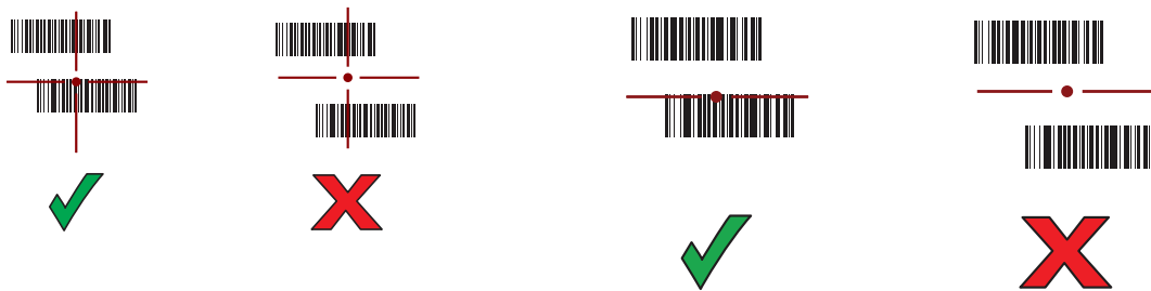
Figure 9 Pick List Mode with Multiple Barcodes in Aiming Pattern: Standard and Extended Range
