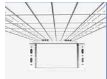
Hanging Cablofil Mounted
