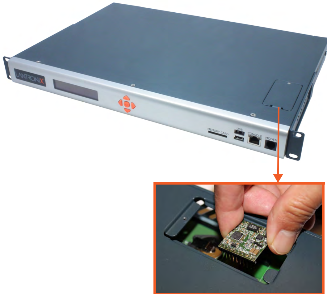
Figure 2-14 Internal Modem Location
