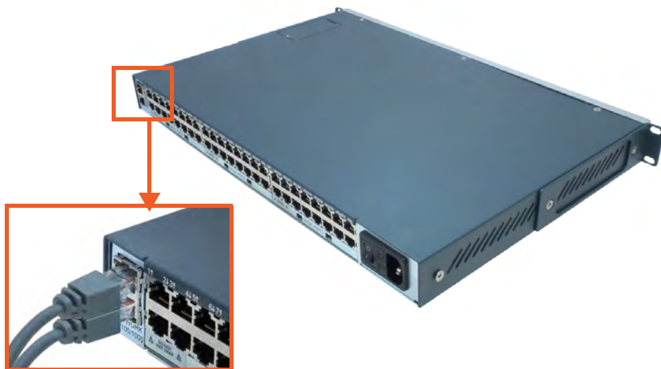
Figure 2-10 Dual Ethernet Network Connection
