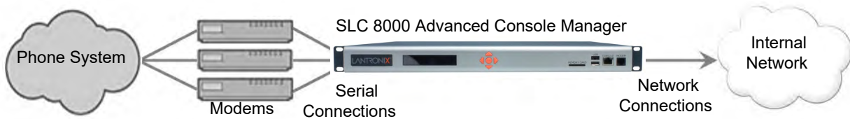
Figure 11-2 Remote Access Server
